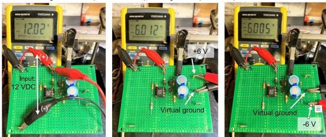
Figure 8. The circuit in Figure 6 is being tested on a universal PCB.
